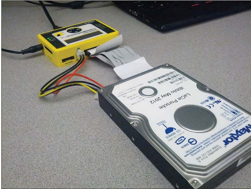
Figure 5: A legacy IDE hard disk connected to a modern forensic write blocker.
